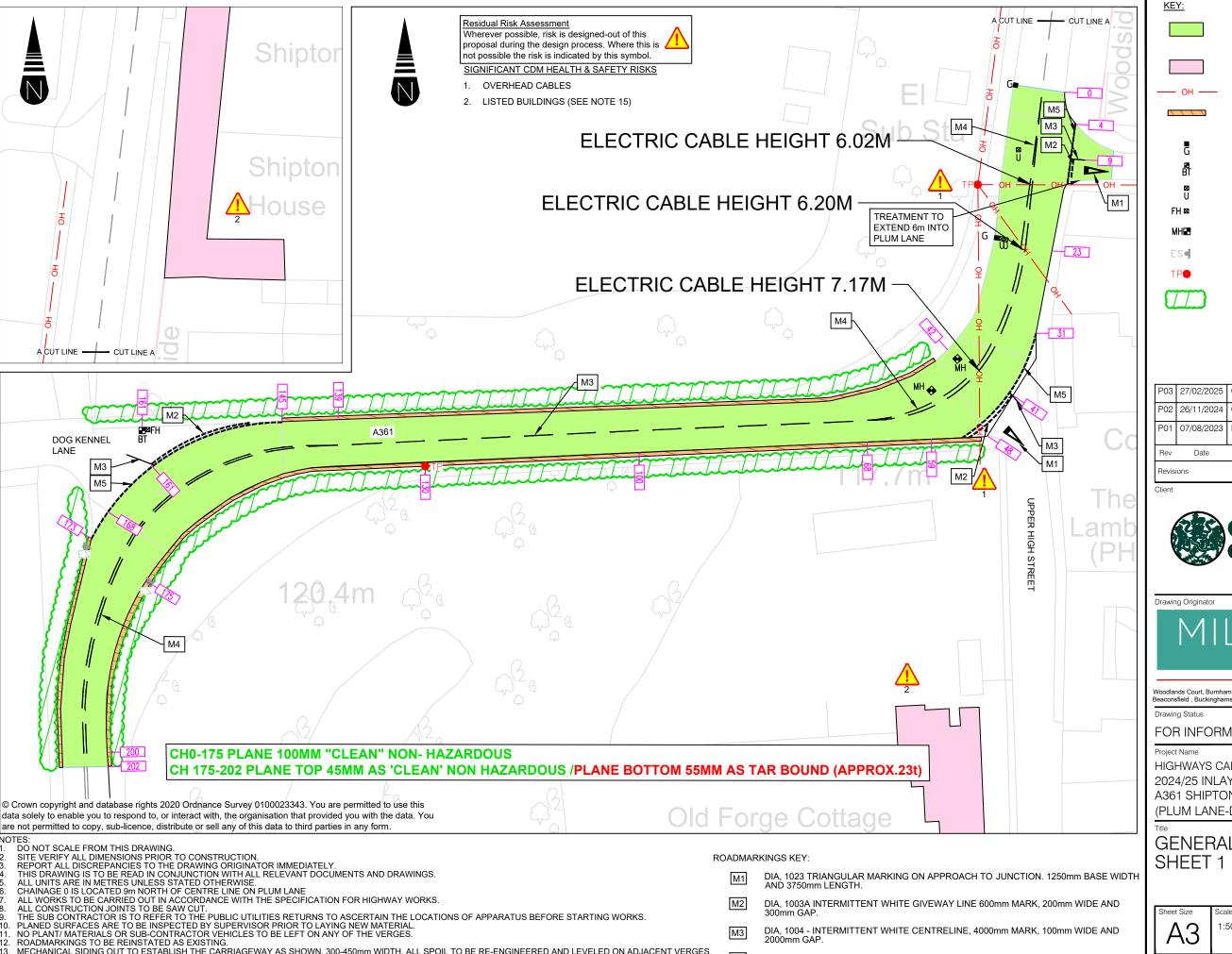
MECHANICAL SIDING OUT TO ESTABLISH THE CARRIAGEWAY AS SHOWN, 300-450mm WIDTH. ALL SPOIL TO BE RE-ENGINEERED AND LEVELED ON ADJACENT VERGES EXISTING GRIPS TO BE RE CUT TO RESTORE DRAINAGE THROUGHOUT. SUPERVISOR TO ENSURE GRIPS LOCATED AT LEAST EVERY 50m.
